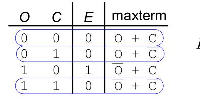
$E = (O + C)(O + \overline{C})(\overline{O} + \overline{C})$  $= \Pi(0, 1, 3)$
